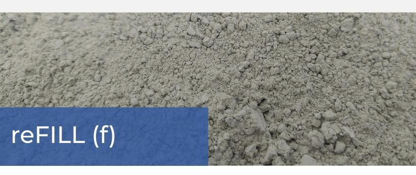
Cost-effective fine epoxy-glass powder filler that can be used as a circular-economy originated filler for various thermoplastic polymers.
